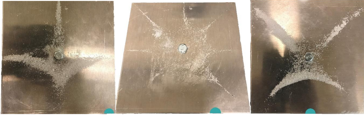
Figure 5 Multiple Chladni patterns created with violin bow. Blue dots mark the spot where the bow was played.
