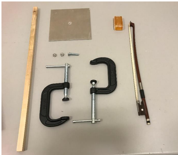
Figure 1 Materials required to set up a Chladni plate with a violin bow. Pictured is a 1/32" violin bow.
