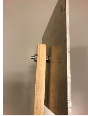
Figure 2 Attach the square dowel to the plate. It should be on tight enough that the plate is firmly in position.
