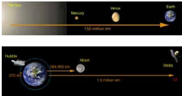
Figure 1. Top: Distance between the Sun and Earth. Bottom: JWST (the Webb) orbits the Sun 1.5 million kilometers away from the Earth at what is called the second Lagrange point or L2. Credit: NASA.
