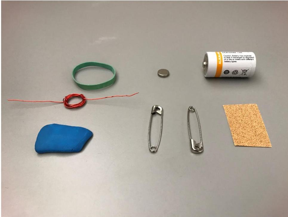
Figure 2 Materials needed for the simple motor.
