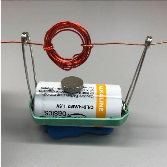
Figure 4 Assembled simple motor. Give it a spin.
