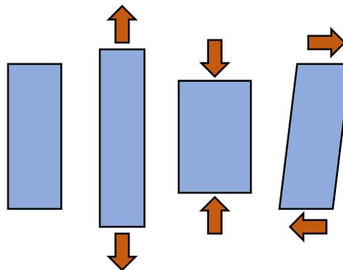
Figure 3: The three main types of stressing forces. From left to right- no stress, tension, compression, and shear.
