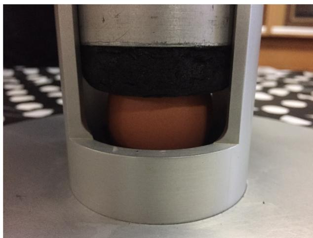
*Figure 2: The proper upright orientation of the egg in the crusher.*
