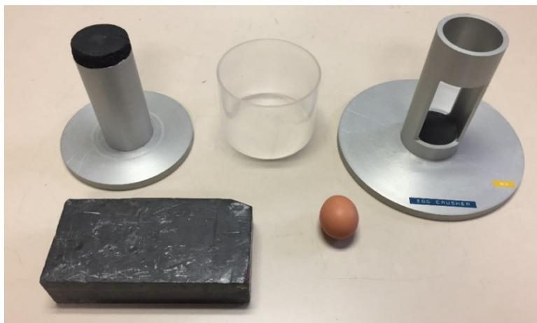
*Figure 1: Egg Crusher apparatus (Aluminum) shown with egg, and one 11 kg weight (~25 lb).*
